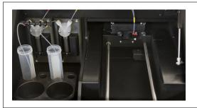
Power OFF the instrument. Push the plate tray to the back of the instrument. Push the read head to the left to create access to the aperture.
