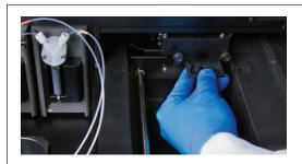
2. Clean the Microplate Sample Tray and Aperture using a soft clean cloth dampened with 70% ethanol. Do **NOT** use other solvents or abrasive cleaners.
