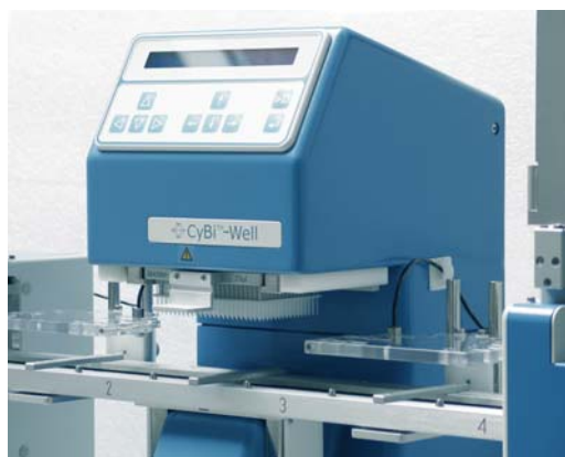
Figure 2. The CyBi®-Well Instrument is a high-precision contact dispenser with simultaneous pipetting capabilities. The instrument also includes a stationary pipetting head (lower picture) with 384 channels, a plate lifter for moving plates up to the tips and a stage for indexing plates to access quadrants in a 1536-well plate. The CyBi®-Well Instrument has a modular design that enables its use as a bench-top pipettor for assay development (for example in addition with stackers or a CyBi® Drop), or it can be incorporated into larger screening systems for higher throughput.
